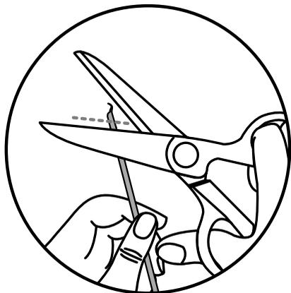
**EN Always snip your ends of the plastic when re-inserting a used strand.**
