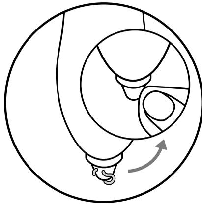
**EN If you have trouble extruding, try cleaning away any plastic that may be stuck to the nozzle while the pen is switched on.**
