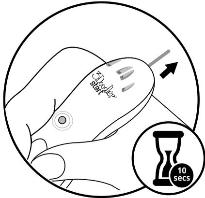
**EN The plastic will reverse for around 10 seconds. The LED light will Quickly FLASH GREEN while reversing.**
