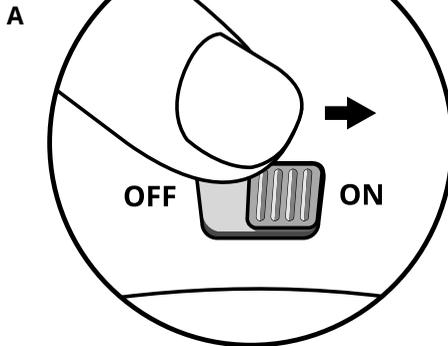
**EN To turn on your 3Doodler Start, slide the power switch from OFF to ON.**
